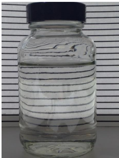
HYPERLAST™ 153/55A Polyol Colourless, clear liquid at 40°C
